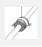
**6. Heavy duty cooling**For heavy duty cooling installations, it is recommended to insulate the seams with tube or sheet insulation as shown in figure 6.
