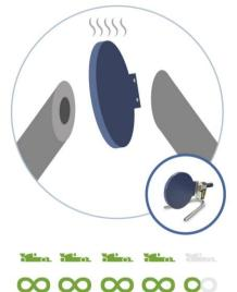
Prefabrication with polyfusion technology (heat plate)
