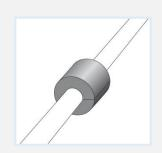
**5. Let glue sit and join**Let glue sit until tack dry (fingernail test) and firmly press the insulation against the pipe hanger insulation block.
