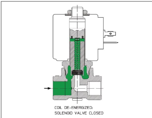
2 way normally closed direct acting solenoid valves have an inlet pipe and a outlet pipe. The plunger, on which a sealing gasket is mounted, provides directly for opening and closing the main orifice. When the coil is not energized the plunger is in such a position as to close the orifice thus preventing the flow of fluid.
