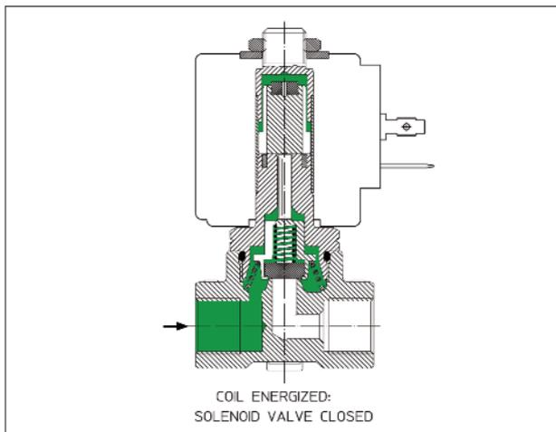
2 way normally open direct acting solenoid valves have an inlet pipe and a outlet pipe. The plunger, acting on the gasket holder by means of a rod, provides for opening and closing the solenoid valve. When the coil is not energized the gasket holder, under the action of a spring, is kept in such a position that the orifice is open, permitting fluid flow.
