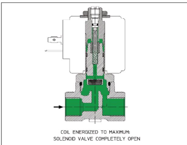
Proportional direct acting solenoid valves have an inlet pipe and a outlet pipe. The plunger, on which a sealing gasket is mounted, provides directly for opening and closing the main orifice of the solenoid valve.
