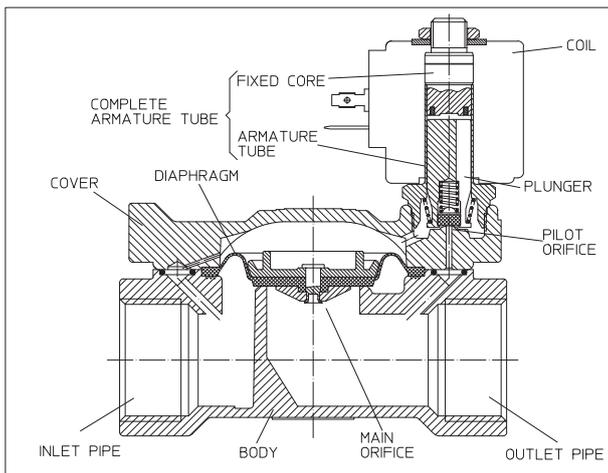
emerge, which may be different depending on the type of coil. (see COIL INDEX). The winding generates the magnetic field while the ferrous-magnetic holder closes the magnetic circuit constituted by the holder itself, the plunger and the fixed core.
