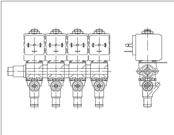
From a functional viewpoint groups of solenoid valves are identical to the singles. The only difference is that they can be put together to form a group of solenoid valves with an inlet pipe and various outlet pipes, each one of which can be opened by energizing the corresponding coil.
