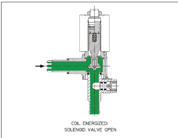
Single solenoid valves for drink-dispenser have an inlet pipe and a outlet pipe on which there is generally a small pipe for attaching a vent. The plunger, on which the sealing cap gasket is fitted, provides directly for opening and closing the orifice, as with two way normally closed solenoid valves.
