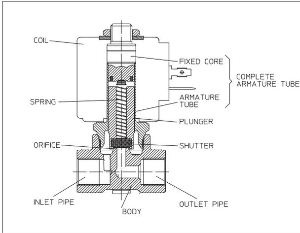
**Fixed core:** component in ferrous-magnetic material which, due to the effect of a magnetic field generated from the coil, attracts the plunger.
