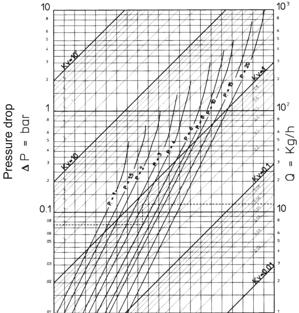
**Example:** Determine the capacity with a loss of load of 750 mm H<sub>2</sub>O and a relative pressure above the solenoid valve of 5 bar with  $Kv=0,8$  m<sup>3</sup>. Starting from the pressure drop value draw an horizontal line until it crosses the absolute pressure  $P_1=5+1=6$  bar, and from this point of intersection, a vertical line to meet the  $Kv$  value 0,8; on the right-hand ordinate you can read the flow rate  $Q=12,8$ .
