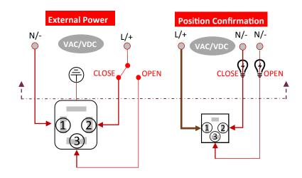
Make the **live (or positive +)** connection to the position confirmation Din plug, pin 1
