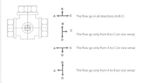
L valve operation: with the handle disassembled is visible, on the stem, a L mark, which indicates the running direction of the ball's holes, allowing the following combinations:
